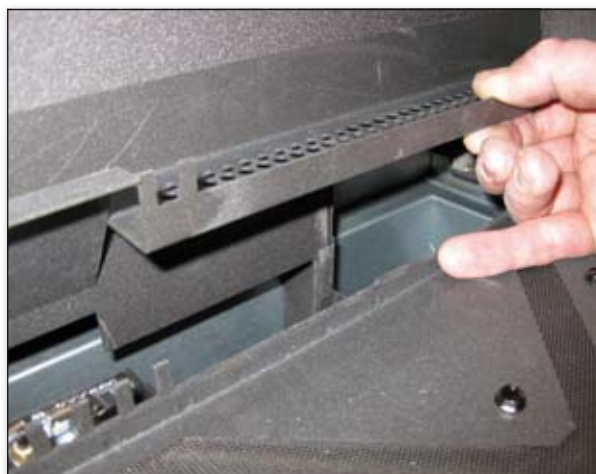
Pay attention to slide in right position and place window (see instruction manual)
